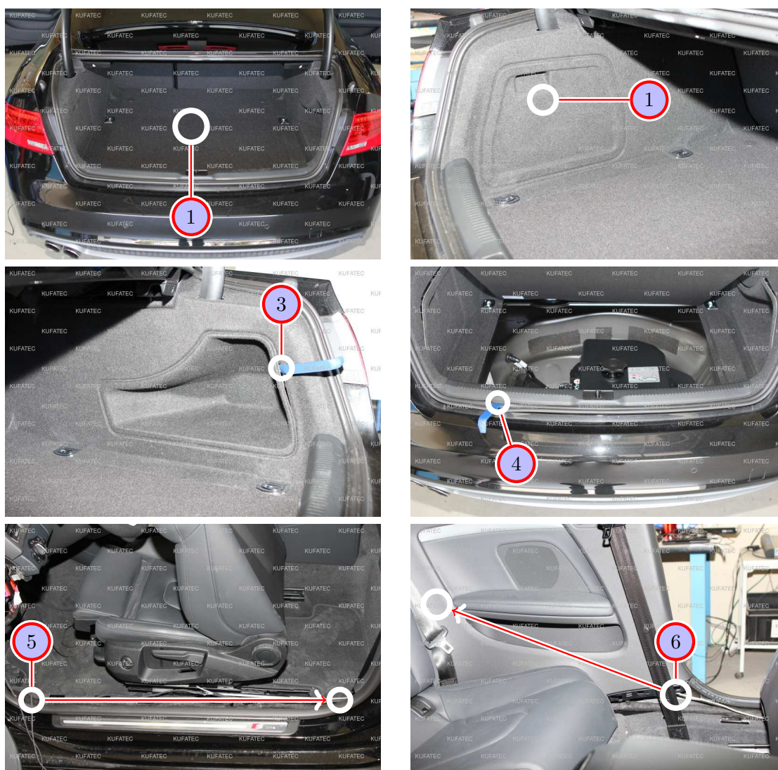
Figure 7: Removing trim panel trunk / cable routing
